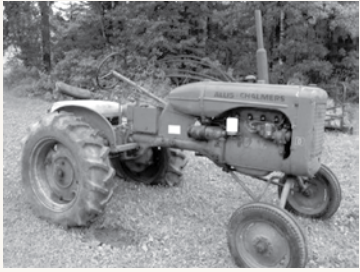
1952 B Allis Chalmers tractor, wide front, 4 cylinder gas, 5 x 24 rear and 4 x 15 front tires, wheel weights & a 6ft. sickle style belly mount mower
