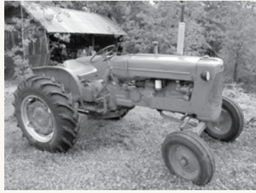
1960 Allis Chalmers D 14 tractor, wide front, 4 cylinder gas, Hi-Lo range, PTO, 13 x 26 rear and 6 x 16 front tires
